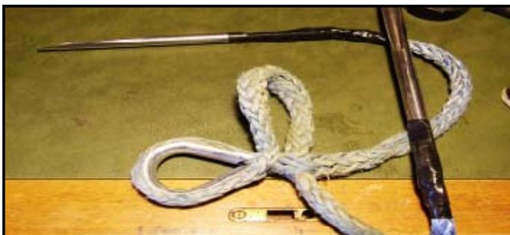
6. Grab the second fid (the one at the end of the rope where it attached to the winch) and repeat the process, as in step 5. Pull tight, at this stage you shouldn't be able to move the thimble and you shouldn't be able to pull the rope out.
