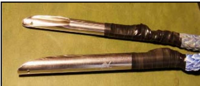
5. Pass the short ended fid through the rope making sure that you don't open any of the strands of fibres but pass by them. This is the tricky part, to make sure that the fitted thimble is tight you will need to adjust the loop so that the opening of the loop is up onto side of the thimble. When you tighten the
