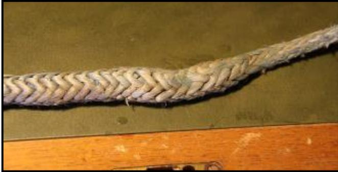
Note: at this stage the rope only has been threaded through itself, so don't unpick any of the individual strands just the whole rope.
